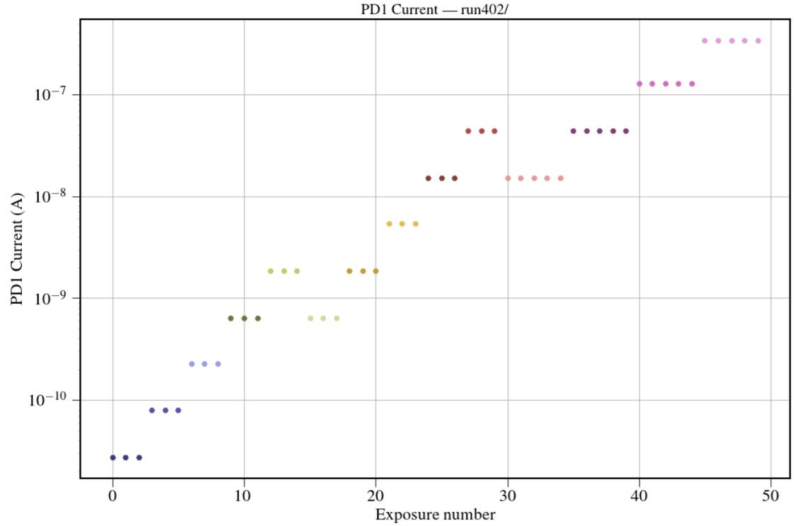
Each point corresponds to an average over a WFI detector (SCA) exposure; each color is a different LED flux
