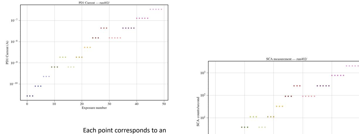
average over a WFI detector (SCA) exposure; each color is a different LED flux
