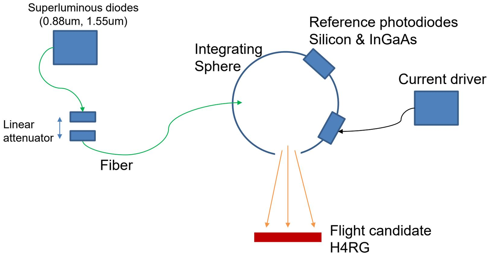
The current plan is to measure CRNL for all flight candidates at 0.88um and 1.55um
