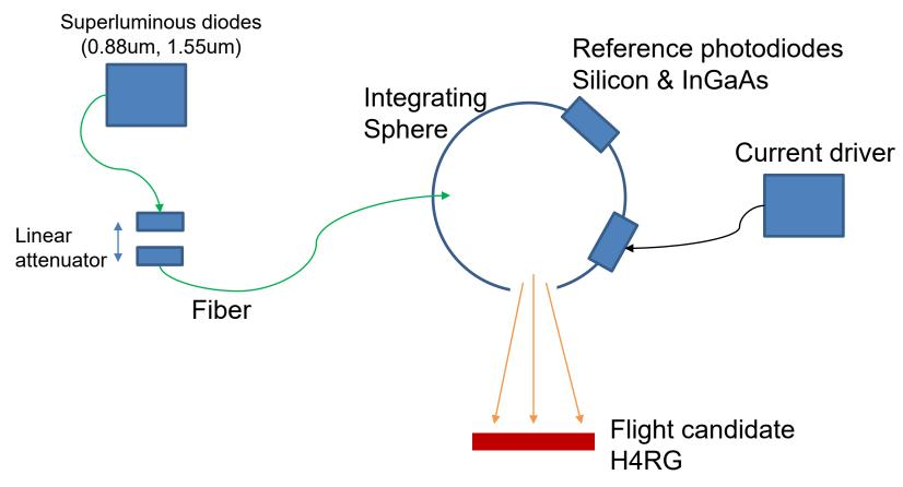
The current plan is to measure CRNL for all flight candidates at 0.88um and 1.55um
