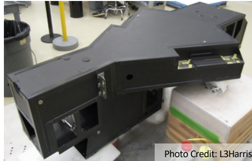
Complete TOMAS—ready for post-cure and thermal cycle
