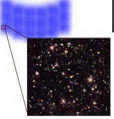
The blue footprint shows a simulated Roman 50-dither WFI exposure. The inset is the size of the Hubble Ultra Deep Field. The Roman field-of-view is more than 100x greater than HST or JWST, facilitating equally sensitive but much wider deep fields.
