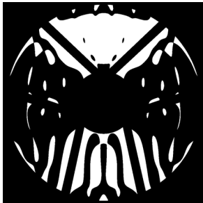
Flight mask designs for the spectroscopy shaped pupil coronagraph. Design by A.J. E. Riggs (JPL).
