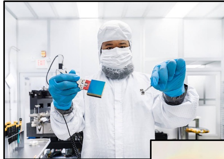
Roman detector compared to cell phone camera
