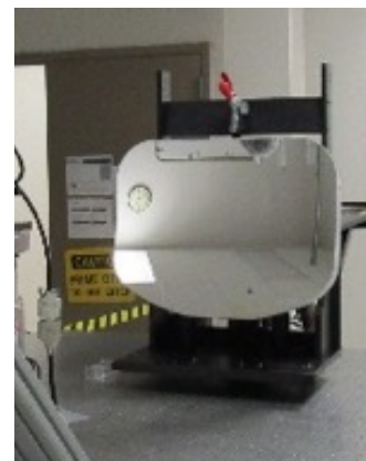
Tertiary Mirror Assembly in ambient optical test
