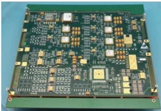
Alignment Drive Electronics Circuit Card Assembly
