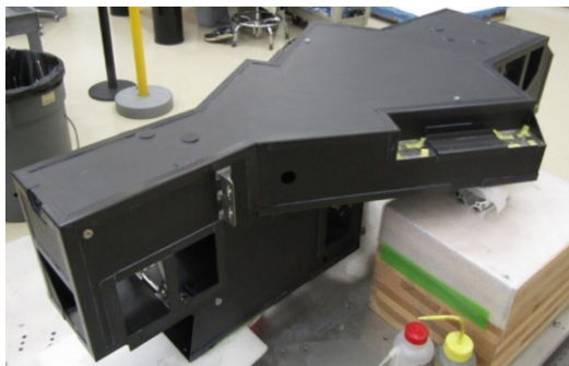
Complete TOMAS—ready for post-cure and thermal cycle
