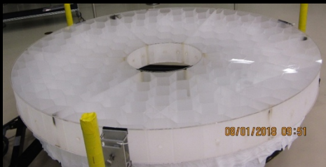
Flight Primary Mirror (SN#3) As received
